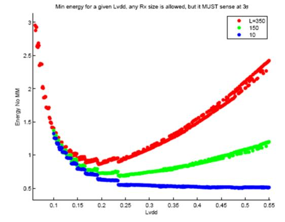
•By designing our own memories, we able to make design decisions based on our needs (small, fast arrays) •By viewing each cell as a small sense amplifier, writes on the cell use a small voltage on the bitlines (3x total savings in a 64x32 array)
